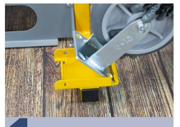
Flip the cart upside down. Install the caster by sliding it under the hook end of the caster mount. Set the caster down into place.
