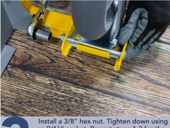
Install a 3/8" hex nut. Tighten down using a 9/16" socket. Repeat steps 1-3 for the remaining casters. Be sure to install both fixed casters on one end, and both swivel casters on the opposite end.
