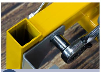
One all four bolts are installed and finger tightened in place, completely tighten them down with a 9/16" wrench and a 9/16" socket.
