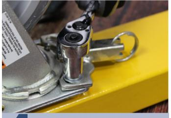
Once all 4 bolts are in place, tighten them securely in place with a wrench.
