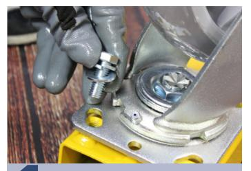
Align a caster over the holes provided. Slide a lock washer, then a 3/4" washer onto a bolt and insert it through the caster and cart body. Finger tighten all of the bolts
