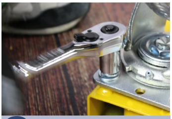
After all 4 bolts are finger tightened, go through and tighten them down with a wrench. Repeat this for THREE of the four casters.
