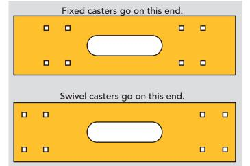
Install the fixed casters on the narrow end and the swivel casters on the wide end.
