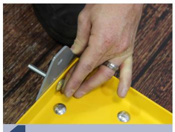
Insert a 2" carriage bolt through the handle bracket.
