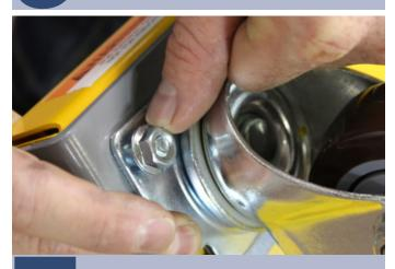
Finger tighten a lock nut onto the bolt.
