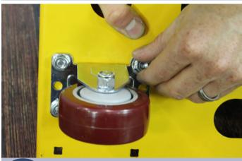
Install the fixed casters in the same manner, but use the 5/8" L bolts. Refer to the diagram on page 2 for placement location. Use a 1/2" socket to tighten.
