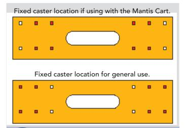
If you intend to use the chair pallet with our Mantis Cart, the fixed casters should be attached using the inner 8 holes.
