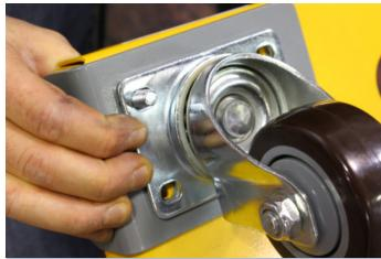
Insert a 3/4" L bolt through the cart, handle bracket and caster.
