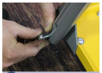
Slide the handle onto the bolt. Finger tighten a nut to hold the handle in place. Repeat with the remaining three bolts.
