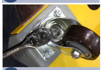
Using a 1/2" socket or wrench, tighten down the bolts. Repeat steps 5-8 for the other swivel caster.
