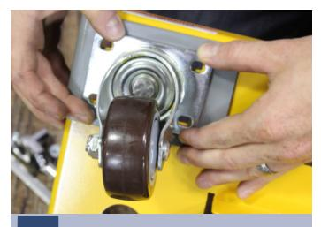
Place a swivel caster onto the handle bracket, aligning the holes.
