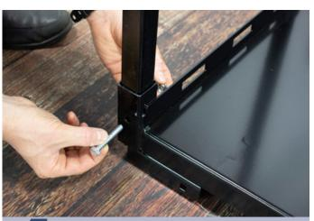
Insert 5/16" x 2" hex bolts (2 total) through the cart base and left end panel. Finger tighten into place. Fully tighten with a 1/2" wrench and socket. Repeat for the right side.
