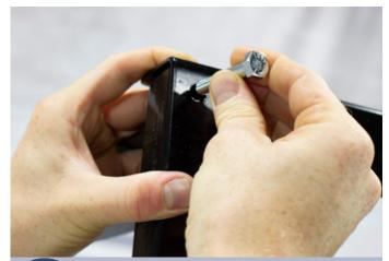
Insert 5/16"x 1-3/4" L hex bolt through the brace and end panels.
