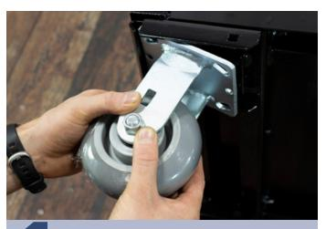
While the cart is still face down, insert a fixed caster into the caster mount on your left side. Insert the second fixed caster in the mount directly below.
