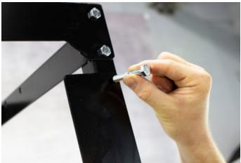
Insert a 5/16"x 1-3/4" L hex bolt through the guard and the end panel. Finger tighten a 5/16" lock nut into place. Do this for all 4 holes on the rear guard.
