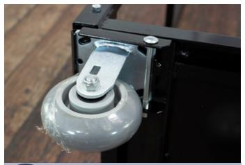
Insert one of the 5" carriage bolts through the caster mount. Finger tighten a 3/8" lock nut to secure the caster in place. Fully tighten with a 9/16" wrench and socket.
