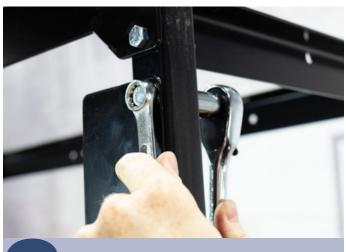
Fully tighten with a 1/2" wrench and socket. Repeat steps 1-3 for the other rear guard.
