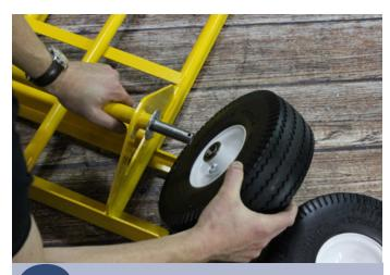
Slide a 3/4" washer followed by a 10" Steel center hub wheel onto the axle.
