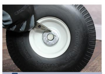
Slide a washer onto the axle. Install the cotter pin and secure it by bending both ends outward with a **needle nose pliers**.
