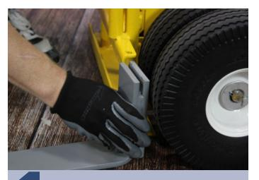
Slide the fork onto the cart frame as shown.
