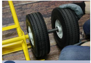
Slide a 10" offset wheel onto the axle, again making sure the offset side is facing towards the body of the cart.
