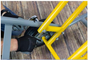
Secure in place using four 3/8" hex bolts and lock nuts. Tighten down using a **9/16"** wrench and socket. Repeat this for the remaining three bolts.
