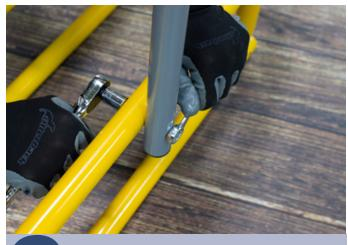
Secure in place using a 3/8" hex bolt and lock nut. Repeat this for the remaining three bolts.
