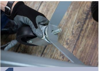
Insert the caster into the mount on the chair lifter bar, then slide a 1/2" washer and a 1/2" lock washer onto the caster.
