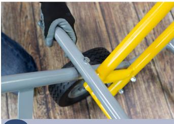
Place the chair stop bar onto the chair lifting bar. Secure into place using two 3/8" hex bolts and lock nuts and a 9/16" wrench and socket.
