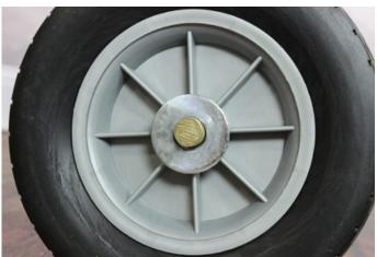
Slide a washer onto the axle.
