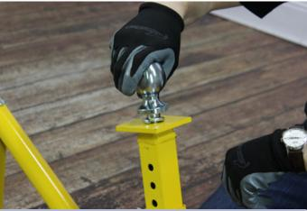
Align the pintle hitch adapter and screw the ball hitch back into place. You may need a 2" wrench to loosen / tighten the ball in place.
