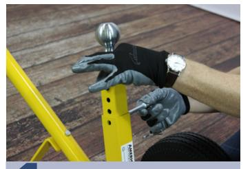
Slide the extension post into the cart frame to the desired height and secure with a 2" snap pin.
