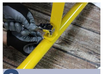
Secure into place using a 5/16" lock nut and a **1/2" wrench and socket**. Repeat steps 2 and 3 to secure the bar in place.
