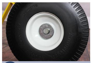
Slide the washer onto the axle.
