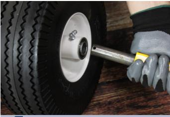
Insert the wheels onto the front axle located towards the bottom of the Multi Mover. The offset side of the wheel should be facing the cart body.
