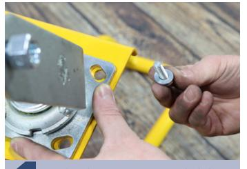
Align the caster mount onto the holes. Place a 5/16" washer onto the 5/16" bolt and insert the bolt through the rear wheel assembly and caster mount.
