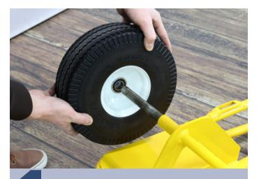
Slide the first wheel onto the axle, making sure the flush side of the hub goes towards the body of the cart.
