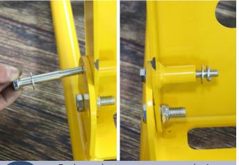
For heavy duty use, we recommend using a bolt kit into the rear wheel assembly. Install a 3/8" washer onto the bolt, then insert the bolt into the rear wheel assembly. Add another 3/8" washer, then a lock washer.
