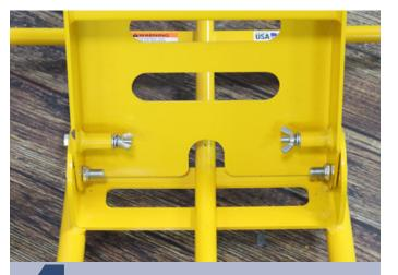
Secure the bolt in place with a wing nut. Repeat the process for the other side.
