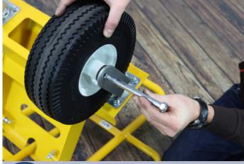
Insert the bushing through one of the wheel hubs, then position the caster wheel into the caster mount.
