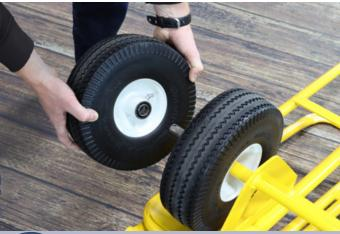
Slide the second wheel onto the axle, this time making sure the offset side faces inward. The offset sides of both tires should be facing each other.
