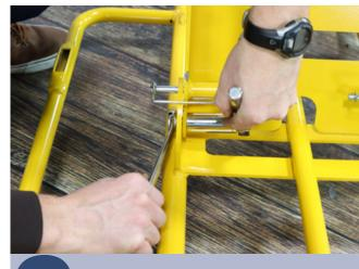
Insert the bolts through the cart body and rear axle assembly. Tighten down with a **3/4**" wrench and ratchet.
