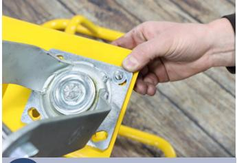
Slide another 5/16" washer onto the bolt,followed by the lock nut. Tighten each nut (but not all the way) with a **1/2" wrench** and a **1/2" socket**.
