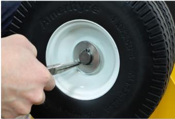
Insert the cotter pin and secure it by bending both ends outward with a **needle nose pliers**. Repeat this process for the other side.
