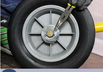
Insert the cotter pin and secure it by bending both ends outward with a **needle nose pliers**.
