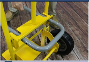
Turn the bar around and slide the rounded end back into the body of the cart.
