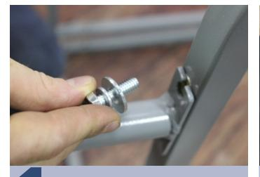
Align the handle over the holes. Slide a lock washer and a washer onto the bolt and insert into the hole.
