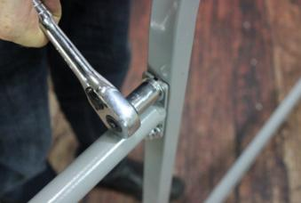
Attach using a 1″ L 5/16″ bolt with a lock washer and standard washer. Tighten down with a 1/2″ socket.
