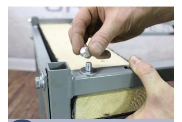
Slide the bolt through the cart frame and carpeted wood. Secure with a 5/16" washer and 5/16" nylon locknut.
