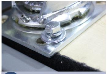
Secure with a 1"L 5/16" bolt, lock washer and standard washer.
