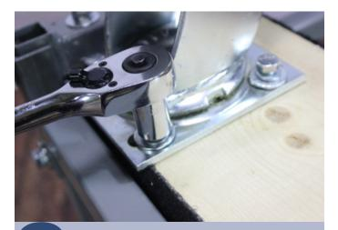
Tighten the bolts down using a 1/2" socket. Repeat steps 1-2 for the remaining casters.
