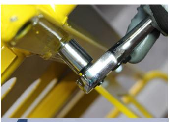
Tighten the nut down with a **9/16"**wrench/socket. Repeat for all bolts.
