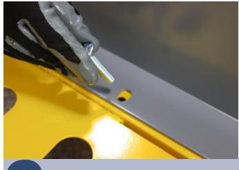
Insert the carriage bolts into the 3 holes.
