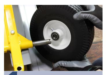
Slide a 10" steel hub wheel onto the front axle. The offset side of the wheel should be facing the cart body.
