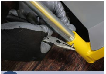
With a **needle nosed pliers** bend the ends of the cotter pin outward, locking the forks in place.
