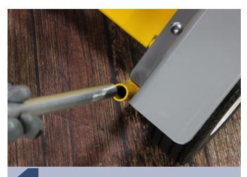
Insert the forks into the fork pockets on the front of the cart.
