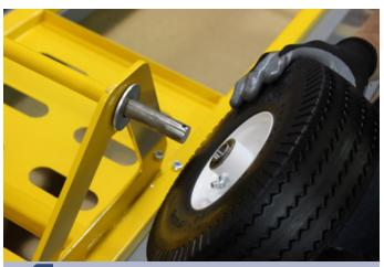
Slide a 3/4" Washer onto rear axle followed by one of the steel hub wheels.
