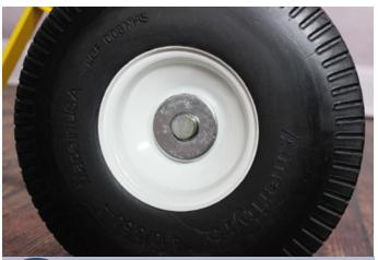
Install a second 3/4" washer onto the wheel.
