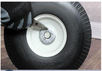
Insert a cotter pin and bend the prongs outward to secure it in place with a **needle nosed pliers**. Repeat steps 1-3 on the other side.
