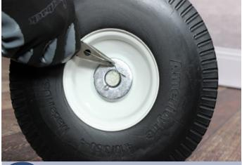
Insert a cotter pin and bend the prongs outward to secure it in place with a **needle nosed pliers**. Repeat steps 1-3 on the other side.
