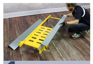
With the cart resting on the axles, align one of the fenders over the cart body.
