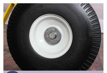
Install a second 3/4" washer onto the wheel.
