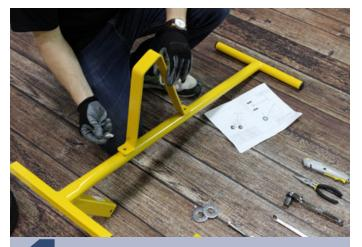
Align the rear leg / bar onto the cart body. The longer leg should be toward the handles, the shorter leg should be toward the axle.
