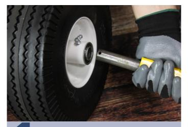
Slide the wheel onto the axle, making sure the offset side is facing inwards, toward the body of the cart.
