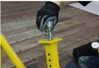
Align the pintle hitch adapter and screw the ball hitch back into place. A 2" wrench may be required to tighten/ loosen the ball.
