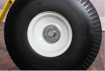
Slide a washer onto the axle.
