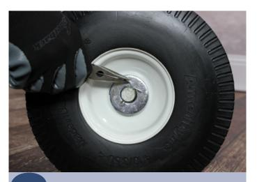
Then insert the cotter pin into the hole provided. Bend the cotter pin outward with a **needle nosed pilers**.
