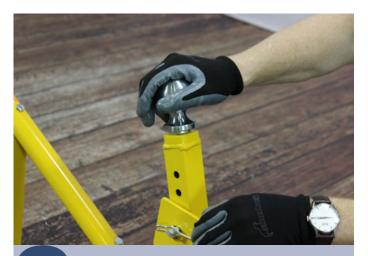
To install the pintle hitch adapter, unscrew the ball from the extension post
